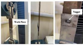
Fig. 13. Tensile test for welded joints
