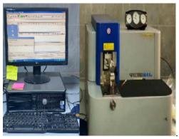
Fig. 2. Optical Emission Spectrometer
